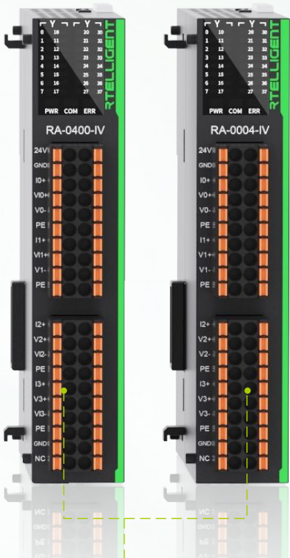
Analog I/O Module • RA-0400-IV: 4-channel analog input, Supports current/voltage input, configurable with different ranges, 16-bit accuracy • RA-0004-IV: 4-channel analog output, Supports current/voltage output, configurable with different ranges, 16-bit accuracy
