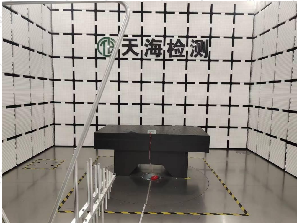
Photographs 2: Set-up for Electrostatic discharge (ESD)
