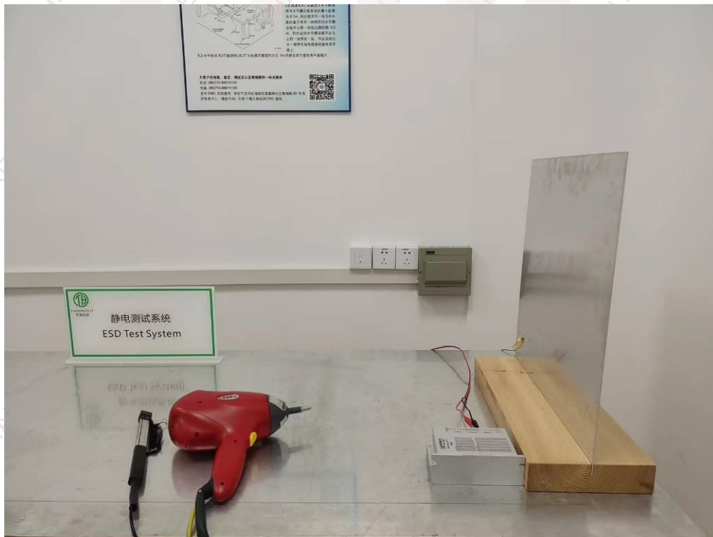
Photographs 2: Set-up for Electrostatic discharge (ESD)
