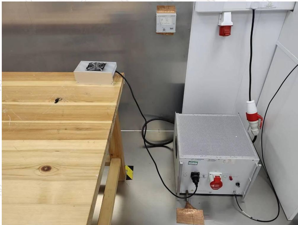
Photograph 2: Set-up for Mains Terminal Continuous Disturbance Voltage
