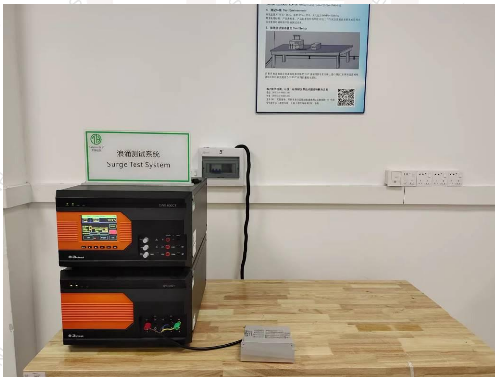
Photograph 6: Set-up for Surge on AC Power Ports
