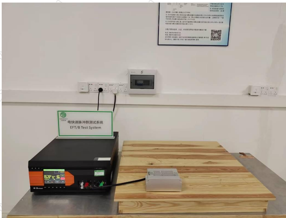
Photograph 6: Set-up for Surge on AC Power Ports
