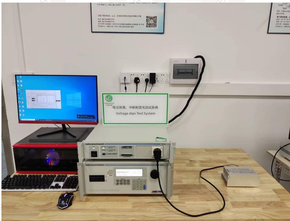
Photograph 8: Set-up for Harmonics & Voltage Dips and Interruptions
