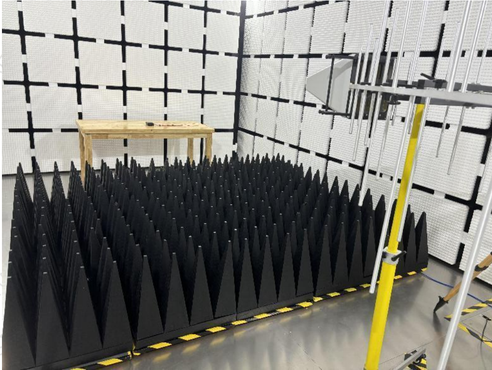
Photograph 3 :Setup for Radio Frequency Electromagnetic Fields
