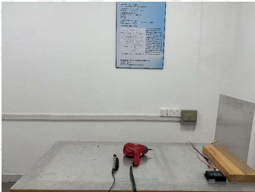
Photograph 2 :Setup for Electrostatic Discharge
