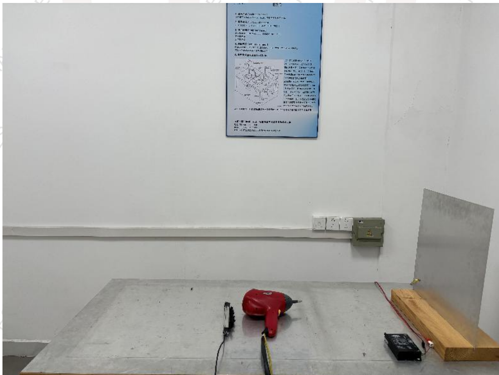
Photograph 2 :Setup for Electrostatic Discharge
