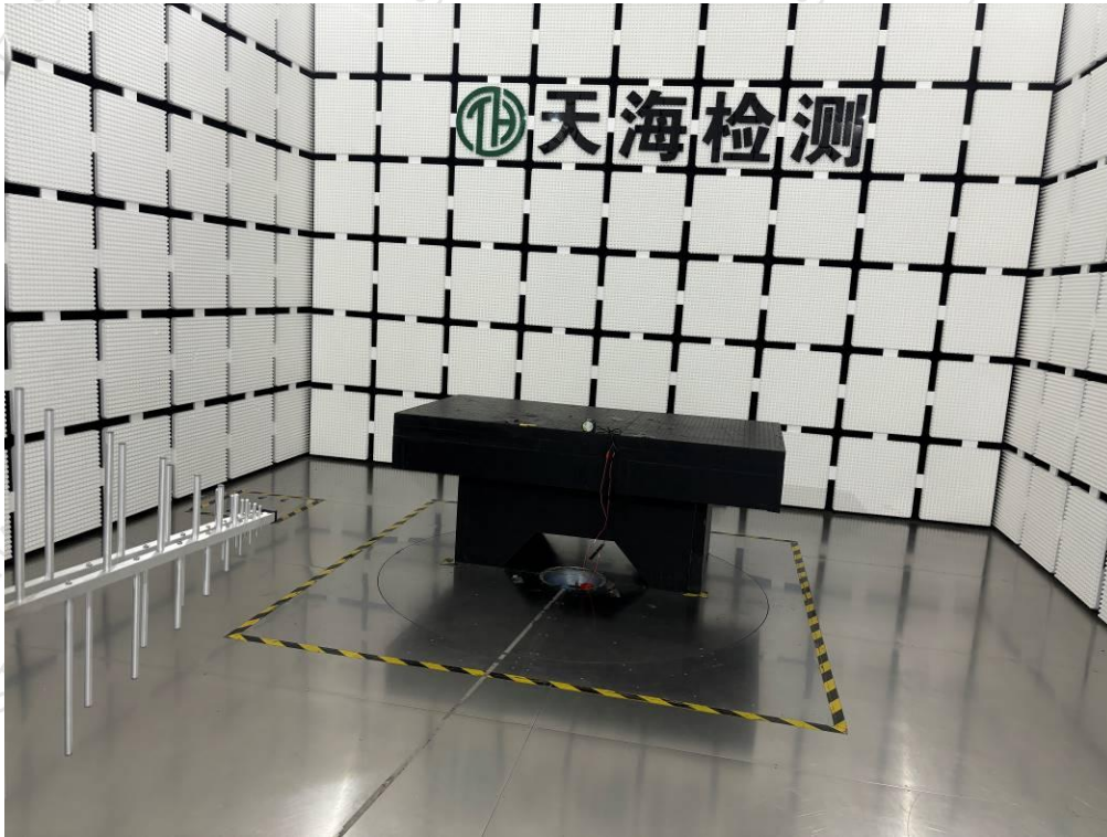
Photograph 1: Setup for Radiated Emission
