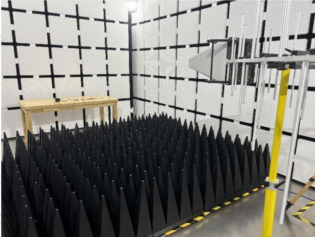
Photograph 3: Setup for Radio Frequency Electromagnetic Fields
