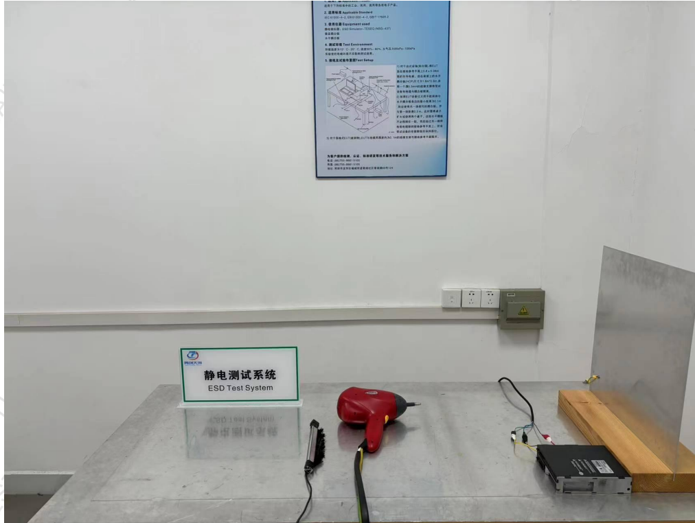
Photograph 3 :Setup for Electrostatic Discharge
