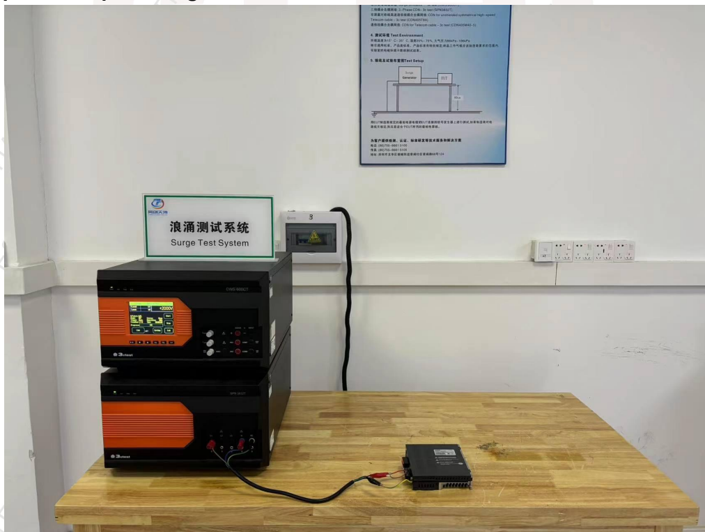
Photograph 6 :Setup for Surge
