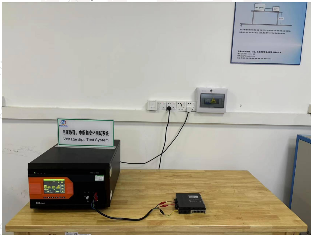
Photograph 8 :Setup for Voltage Dips And Interruptions
