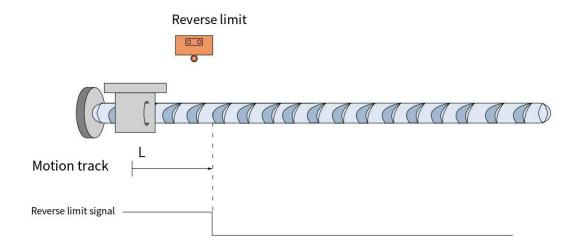
When NOT=ON, it starts homing at a low speed in the forward direction and stops when it encounters the falling edge of NOT.
