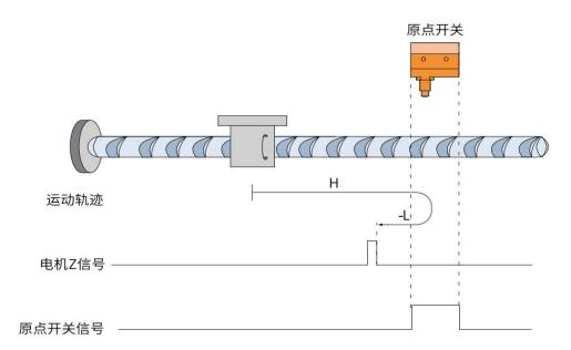
When HOME=OFF, it starts homing at a high speed in the forward direction. When encountering the rising edge of HOME, it slows down in the reverse
