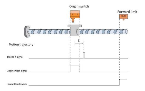
When HOME=ON and POT=OFF, the machine starts homing at a low forward speed and stops at the first Z signal after the falling edge of HOME.
