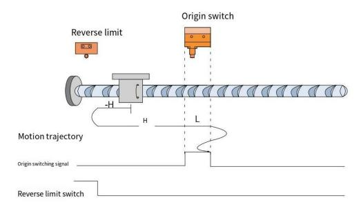
When HOME=OFF, NOT=OFF, it starts homing at high speed in the reverse direction. After encountering the rising edge of NOT, it automatically runs in the
