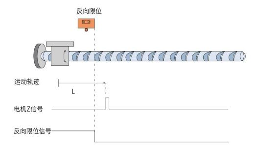
When NOT=ON, it starts homing, directly returning homing at a low speed in the forward direction, and stops at the first Z signal after encountering the NOT falling edge.
