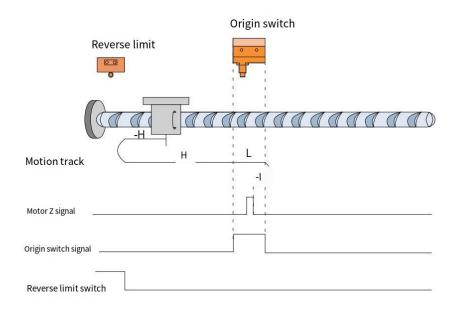
When HOME=OFF, NOT=OFF, it starts homing at high speed in the reverse direction. After encountering the rising edge of NOT, it immediately runs in the forward direction at high speed. After encountering the rising edge of HOME, it runs in the forward direction at low speed. After encountering the falling edge of
