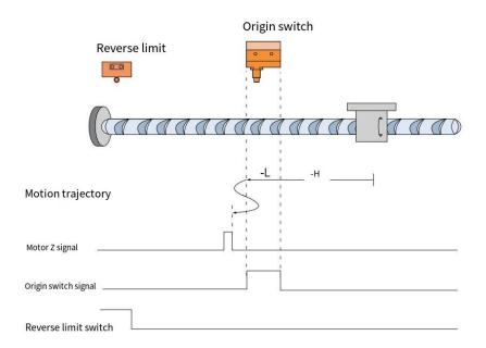
When HOME=ON, NOT=OFF, it starts homing at a low speed in the reverse direction. After encountering the falling edge of HOME, it decelerates and reverses, runs at a low speed in the forward direction, and stops at the first Z signal after the rising edge of HOME.
