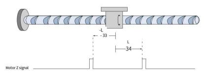
Zero return method 33: Run in reverse at low speed and stop at the first Z signal.
