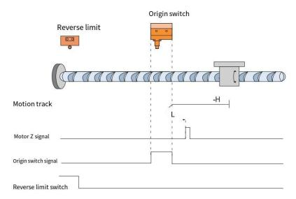
When HOME=OFF, NOT=OFF, it starts homing at high speed in the reverse direction. After encountering the rising edge of HOME, it decelerates and reverses, runs at low speed in the forward direction, and stops when encountering the first Z signal of the falling edge of HOME.
