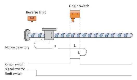
When HOME=OFF, NOT=OFF, it starts homing at high speed in the reverse direction. After encountering the rising edge of NOT, it automatically runs in the forward direction at high speed. After encountering the rising edge of HOME, it runs in the forward direction at low speed. After encountering the falling edge of
