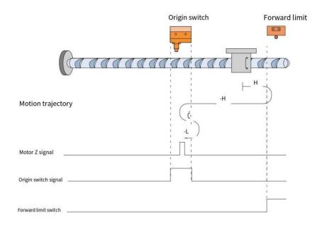
When HOME=OFF, POT=OFF, it starts homing at high speed in the forward direction. After encountering the rising edge of POT, it automatically runs in the reverse direction at high speed. After encountering the rising edge of HOME, it decelerates and reverses, and runs at low speed in the forward direction. After encountering the falling edge of HOME, it decelerates and reverses, and runs at low speed in the reverse direction. It stops at the first Z signal after the rising edge of HOME.
