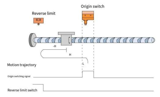
When HOME=OFF, NOT=OFF, it starts homing at high speed in the reverse direction. After encountering the rising edge of NOT, it automatically runs in the forward direction at high speed. After encountering the rising edge of HOME, it decelerates and reverses, and runs in the reverse direction at low speed. After encountering the falling edge of HOME, it decelerates and reverses, and runs in the forward direction at low speed. It stops after encountering the rising edge of HOME again.
