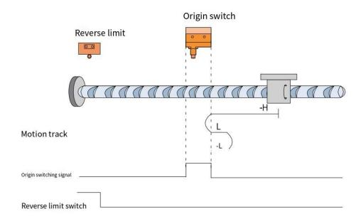
When HOME=OFF, NOT=OFF, it starts homing at high speed in the reverse direction. After encountering the rising edge of HOME, it decelerates and reverses, and runs at low speed in the forward direction. After encountering the falling edge of HOME, it decelerates and reverses, and runs at low speed in the reverse direction. It stops after encountering the rising edge of HOME again.
