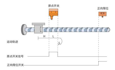
When HOME=OFF, POT=OFF, it starts homing at high speed in the forward direction. After encountering the rising edge of HOME, it runs at low speed in the forward direction. After encountering the falling edge of HOME, it decelerates and reverses, runs at low speed in the reverse direction, and stops after encountering the rising edge of HOME.
