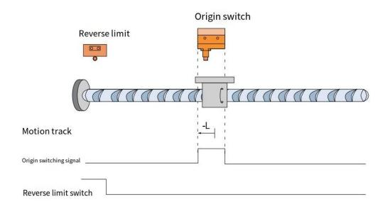
When HOME=ON, NOT=OFF, it starts homing at a low speed in the reverse direction. After encountering the falling edge of HOME, it decelerates and reverses, runs at a low speed in the forward direction, and stops after encountering the rising edge of HOME.
