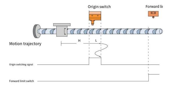
When HOME=OFF, POT=OFF, it starts homing at high speed in the forward direction. After encountering the rising edge of HOME, it runs at low speed in the forward direction. After encountering the falling edge of HOME, it decelerates and reverses, and runs at low speed in the reverse direction. After encountering the rising edge of HOME, it decelerates and reverses, and runs at low speed in the forward direction. It stops after encountering the falling edge of HOME again.
