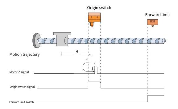
When HOME=OFF, POT=OFF, it starts to homing at high speed in the forward direction. After encountering the rising edge of HOME, it decelerates and reverses, and runs at low speed in the reverse direction. After encountering the falling edge of HOME, it decelerates and reverses, and runs at low speed in the forward direction. It stops at the first Z signal after the rising edge of HOME.
