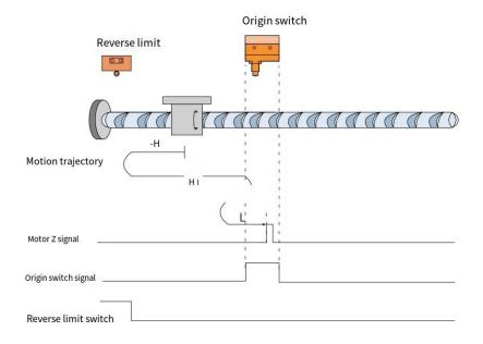
When HOME=OFF, NOT=OFF, it starts homing at high speed in the reverse direction. After encountering the rising edge of NOT, it immediately runs in the forward direction at high speed. After encountering the rising edge of HOME, it decelerates and reverses, and runs in the reverse direction at low speed. After encountering the falling edge of HOME, it decelerates and reverses, and runs in the forward direction at low speed. It stops at the first Z signal after the rising edge of HOME.
