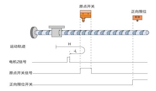
When HOME=OFF and POT=OFF, the homing process starts. It begins moving at high speed in the positive direction. After encountering the rising edge of the HOME signal, it decelerates and reverses direction, then continues moving at low speed in the reverse direction. It stops at the first Z signal encountered after the falling edge of the HOME signal.
