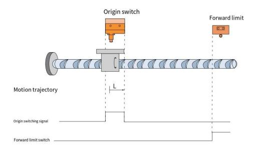
When HOME=ON and POT=OFF, the system starts homing at a low forward speed and stops when it encounters the falling edge of HOME.
