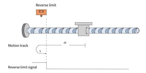
When NOT=OFF, it starts homing at a high speed in the reverse direction. After encountering the rising edge of NOT, it decelerates and reverses, runs at a low speed in the forward direction, and stops after encountering the falling edge of NOT.
