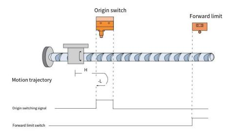
When HOME=OFF, POT=OFF, it starts homing at high speed in the forward direction. After encountering the rising edge of HOME, it decelerates and reverses, runs at low speed in the reverse direction, and stops when encountering the falling edge of HOME.
