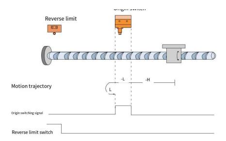
When HOME=OFF, NOT=OFF, it starts homing at high speed in the reverse direction. After encountering the rising edge of HOME, it runs in the reverse direction at low speed. After encountering the falling edge of HOME, it decelerates and reverses, runs in the forward direction at low speed, and stops after encountering the rising edge of HOME.
