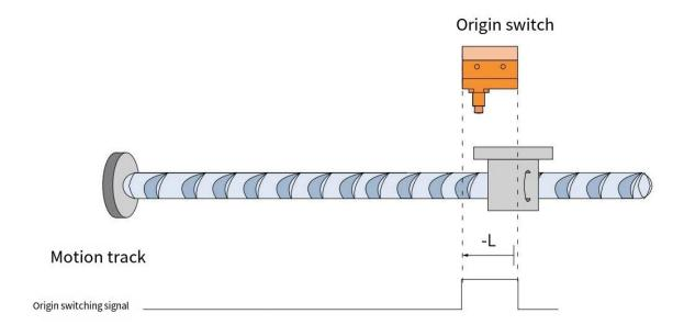
When HOME=ON, the machine starts homing at a low speed in the reverse direction and stops when it encounters the falling edge of HOME.
