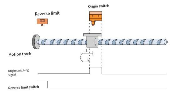
When HOME=ON, NOT=OFF, it starts homing at a low speed in the forward direction. After encountering the falling edge of HOME, it decelerates and reverses, running at a low speed in the forward direction, and stops after encountering the rising edge of HOME.
