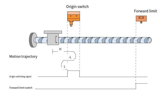
When HOME=OFF, POT=OFF, it starts homing at high speed in the forward direction. After encountering the rising edge of HOME, it decelerates and reverses, and runs at low speed in the reverse direction. After encountering the falling edge of HOME, it decelerates and reverses, and runs at low speed in the forward direction. It stops after encountering the rising edge of HOME again.
