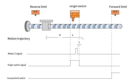
When HOME=OFF, POT=OFF, it starts homing at high speed in the forward direction. After encountering the rising edge of HOME, it runs at low speed in the forward direction. After encountering the falling edge of HOME, it decelerates and reverses, runs at low speed in the reverse direction, and stops at the first Z signal after the rising edge of HOME.
