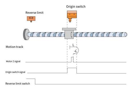
When HOME=ON, NOT=OFF, it starts homing at a low speed in the forward direction. After encountering the falling edge of HOME, it decelerates and reverses, running at a low speed in the reverse direction. It stops at the first Z signal after the rising edge of HOME.
