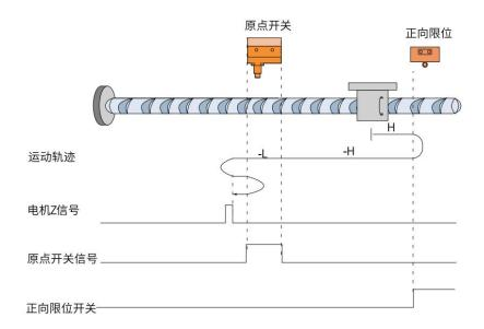
When HOME=OFF and POT=OFF, the homing process begins. It starts moving at high speed in the positive direction. Upon detecting the rising edge of the POT signal, it automatically reverses direction and moves at high speed in the negative direction. After encountering the rising edge of the HOME signal, it switches to low-speed reverse movement.
