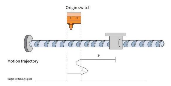
When HOME=OFF, it starts homing at a high speed in the reverse direction. After encountering the rising edge of HOME, it decelerates and reverses, and runs at a low speed in the forward direction. After encountering the falling edge
