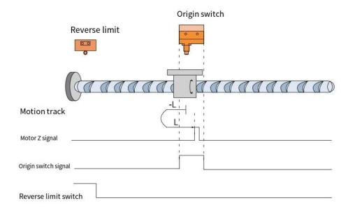
When HOME=ON, NOT=OFF, it starts homing at a low speed in the forward direction. After encountering the falling edge of HOME, it decelerates and reverses, running at a low speed in the forward direction. It stops at the first Z signal after the rising edge of HOME.
