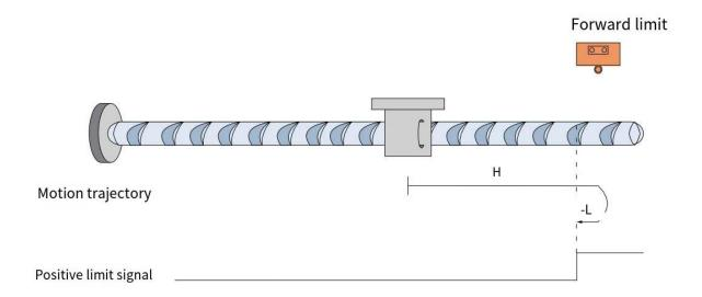
When POT=OFF, it starts homing at a high forward speed. After encountering the rising edge of POT, it decelerates and reverses, runs at a low speed in the reverse direction, and stops after encountering the falling edge of POT.
