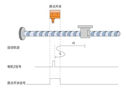
When HOME=OFF, it starts homing at high speed in reverse. When encountering the rising edge of HOME, it slows down in reverse and runs at low speed in forward direction. When encountering the falling edge of HOME, it slows down in reverse and runs at low speed in reverse direction. The first Z signal after encountering the rising edge of HOME stops the machine.
