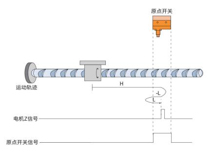
When HOME=OFF, it starts homing at a high speed in the forward direction. When encountering the rising edge of HOME, it slows down in the reverse
