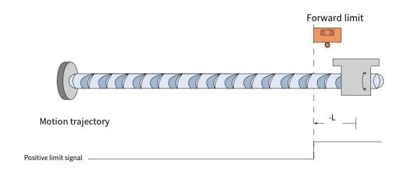
When POT=ON, it starts homing at a low speed in the reverse direction and stops when it encounters the falling edge of POT.
