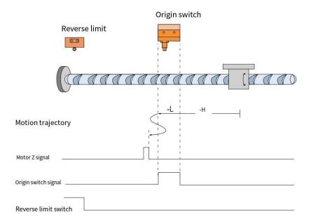
When HOME=OFF, NOT=OFF, it starts homing at high speed in the reverse direction. After encountering the rising edge of HOME, it runs in the reverse direction at low speed. After encountering the falling edge of HOME, it decelerates and reverses, runs in the forward direction at low speed, and stops at the first Z signal after the rising edge of HOME.
