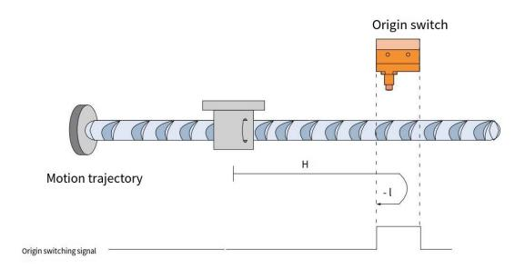
When HOME=OFF, it starts homing at high speed in the forward direction. After encountering the rising edge of HOME, it decelerates and reverses, runs at low speed in the reverse direction, and stops after encountering the falling edge of HOME.
