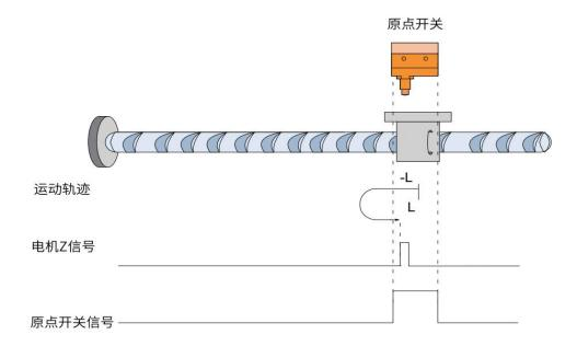
When HOME=ON, it starts homing at low speed in reverse. When encountering the NOT falling edge, it slows down in reverse and runs at low speed in forward direction. When encountering the HOME rising edge, the first Z signal stops the machine.
