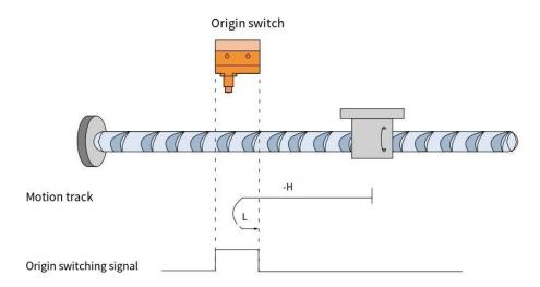
When HOME=OFF, it starts homing at a high speed in the reverse direction. After encountering the rising edge of HOME, it decelerates and reverses, runs at a low speed in the forward direction, and stops after encountering the falling edge of HOME.
