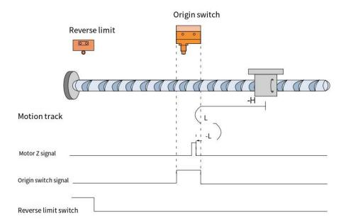
When HOME=OFF, NOT=OFF, it starts homing at high speed in the reverse direction. After encountering the rising edge of HOME, it decelerates and reverses, and runs at low speed in the forward direction. After encountering the falling edge of HOME, it decelerates and reverses, and runs at low speed in the reverse direction. It stops at the first Z signal after the rising edge of HOME.
