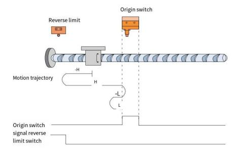
When HOME=OFF, NOT=OFF, it starts homing at high speed in the reverse direction. After encountering the rising edge of NOT, it automatically runs in the forward direction at high speed. After encountering the rising edge of HOME, it decelerates and reverses, and runs in the reverse direction at low speed. After encountering the falling edge of HOME, it decelerates and reverses, and runs in the forward direction at low speed. It stops after encountering the rising edge of HOME again.
