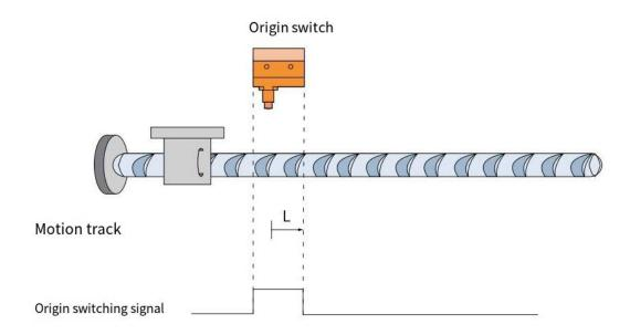
When HOME=ON, it starts homing at a low speed in the forward direction and stops when it encounters the falling edge of HOME.
