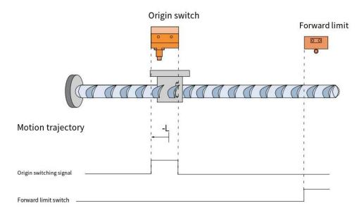
When HOME=ON and POT=OFF, the machine starts homing at a low speed in the reverse direction and stops when it encounters the falling edge of HOME.
