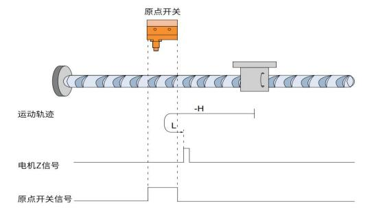
When HOME=OFF, start homing at reverse high speed. When encountering the rising edge of HOME, slow down in reverse and run at low speed in forward direction. Stop at the first Z signal after encountering the falling edge of HOME.
