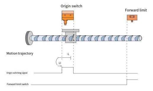
When HOME=ON and POT=OFF, it starts homing at a low speed in the reverse direction. After encountering the falling edge of HOME, it decelerates and reverses, runs at a low speed in the forward direction, and stops after encountering the rising edge of HOME.
