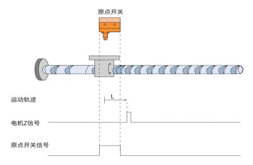
When HOME=ON, it starts homing at a low forward speed, and stops at the first Z signal after encountering the falling edge of HOME.
