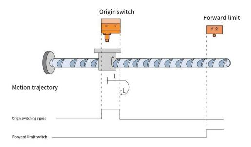
When HOME=ON and POT=OFF, the machine starts homing at a low speed in the forward direction. After encountering the falling edge of HOME, it decelerates and reverses, runs at a low speed in the reverse direction, and stops after encountering the rising edge of HOME.
