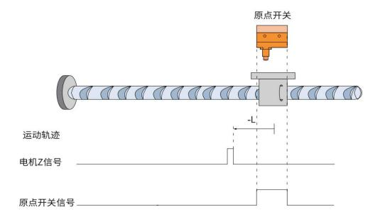
When HOME=ON, it starts **homing**, starting **homing at** low reverse speed, and stopping at the first Z signal after encountering the falling edge of HOME.
