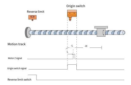
When HOME=OFF, NOT=OFF, it starts homing at high speed in the reverse direction. After encountering the rising edge of HOME, it runs in the reverse direction at low speed. After encountering the falling edge of HOME, it decelerates and reverses, runs in the forward direction at low speed, and stops at the first Z signal after the rising edge of HOME.
