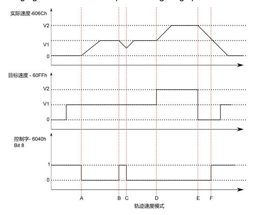
The above figure shows the corresponding relationship between the motor operating status, actual speed, target speed, and control word.
