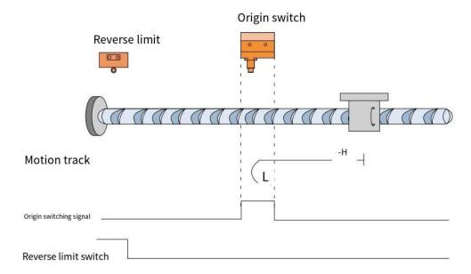
When HOME=OFF, NOT=OFF, it starts homing at high speed in the reverse direction. After encountering the rising edge of HOME, it decelerates and reverses, runs at low speed in the forward direction, and stops when encountering the falling edge of HOME.
