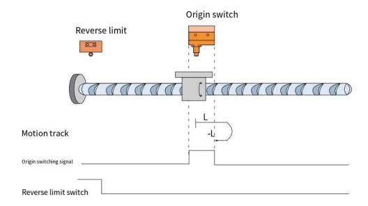
When HOME=ON, NOT=OFF, it starts homing at a low speed in the forward direction. After encountering the falling edge of HOME, it decelerates and reverses, runs at a low speed in the reverse direction, and stops after encountering the rising edge of HOME.
