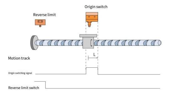
When HOME=ON, NOT=OFF, the system starts homing at a low forward speed and stops when it encounters the falling edge of HOME.
