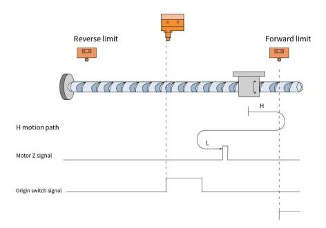
When HOME=OFF, POT=OFF, it starts homing at high speed in the forward direction. After encountering the rising edge of POT, it automatically runs in the reverse direction at high speed. After encountering the rising edge of HOME, it decelerates and reverses, runs in the forward direction at low speed, and stops at the first Z signal after the falling edge of HOME.
