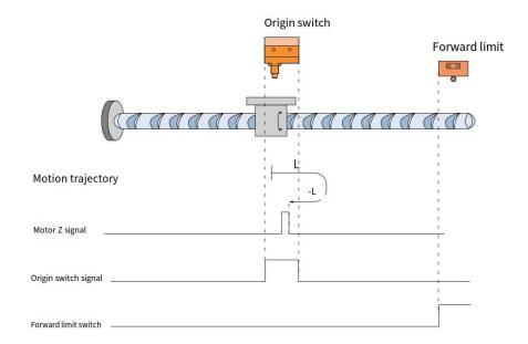
When HOME=ON, POT=OFF, it starts homing at a low speed in the forward direction. After encountering the falling edge of HOME, it decelerates and reverses, runs at a low speed in the reverse direction, and stops at the first Z signal after the rising edge of HOME.
