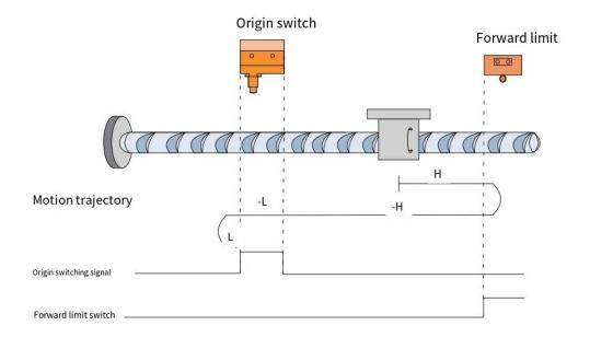
When HOME=OFF, POT=OFF, it starts homing at high speed in the forward direction. When it encounters the rising edge of POT, it automatically runs in the reverse direction at high speed. When it encounters the rising edge of HOME, it runs in the reverse direction at low speed. When it encounters the falling edge of HOME, it decelerates and reverses, runs in the forward direction at low speed, and stops when it encounters the rising edge of HOME.
