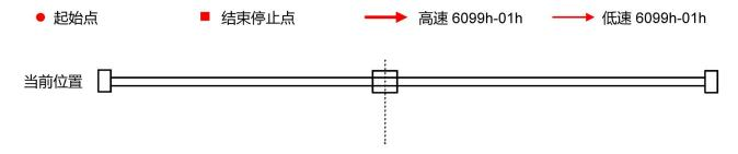
Return to zero method 35, using the current position as the mechanical origin.
