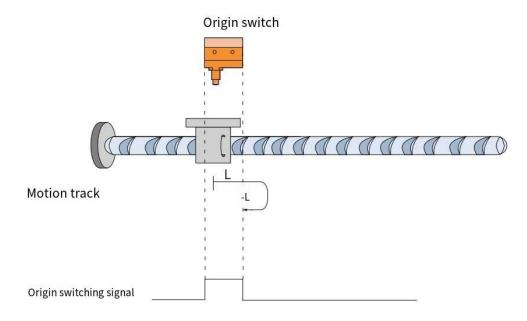
When HOME=ON, it starts homing at a low speed in the forward direction. After encountering the falling edge of HOME, it decelerates and reverses, runs at a low speed in the reverse direction, and stops after encountering the rising edge of HOME.
