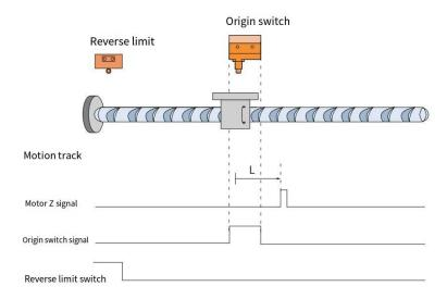
When HOME=ON, NOT=OFF, the machine starts homing at a low forward speed and stops at the first Z signal after the falling edge of HOME.
