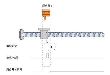
When HOME=ON, it starts homing at a low speed in the forward direction. When encountering the descending edge of HOME, it slows down in the reverse direction and runs at a low speed in the reverse direction. When encountering the rising edge of HOME, the first Z signal stops the machine.
