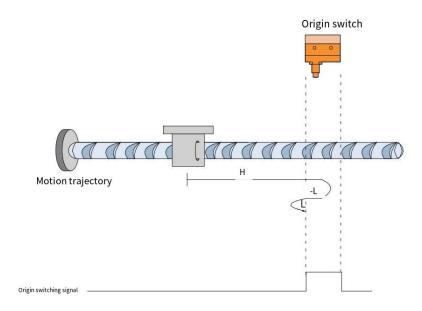
When HOME=OFF, it starts homing at a high forward speed. After encountering the rising edge of HOME, it decelerates and reverses, and runs at a low speed in the reverse direction. After encountering the falling edge of HOME, it decelerates and reverses, and runs at a low forward speed. It stops after encountering the rising edge of HOME again.
