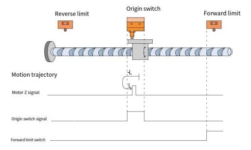
When HOME=ON and POT=OFF, the machine starts homing at a low speed in the reverse direction. After encountering the falling edge of HOME, it decelerates and reverses, and runs at a low speed in the forward direction. It stops at the first Z signal after the rising edge of HOME.
