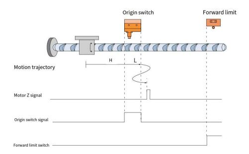
When HOME=OFF, POT=OFF, it starts homing at high speed in the forward direction. After encountering the rising edge of HOME, it runs at low speed in the forward direction. After encountering the falling edge of HOME, it decelerates and reverses, and runs at low speed in the reverse direction. After encountering the rising edge of HOME, it decelerates and reverses, and runs at low speed in the forward direction. It stops at the first Z signal after the falling edge of HOME.
