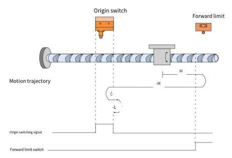
When HOME=OFF, POT=OFF, it starts homing at high speed in the forward direction. After encountering the rising edge of POT, it automatically runs in the reverse direction at high speed. After encountering the rising edge of HOME, it decelerates and reverses, and runs in the forward direction at low speed. After encountering the falling edge of HOME, it decelerates and reverses, and runs in the reverse direction at low speed. It stops after encountering the rising edge of HOME again.
