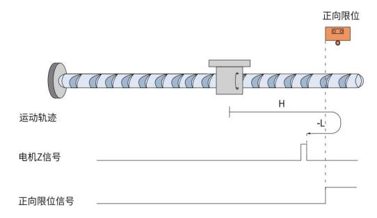
When POT=OFF, start homing at high speed in the forward direction. When encountering the rising edge of POT, slow down, reverse, and run at low speed in the reverse direction
