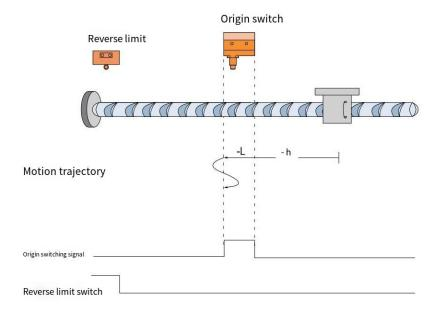
When HOME=OFF, NOT=OFF, it starts homing at high speed in the reverse direction. After encountering the rising edge of HOME, it runs in the reverse direction at low speed. After encountering the falling edge of HOME, it decelerates and reverses, runs in the forward direction at low speed, and stops after encountering the rising edge of HOME.
