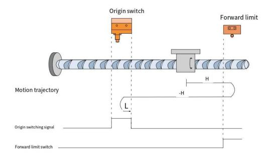
When HOME=OFF, POT=OFF, it starts homing at high speed in the forward direction. After encountering the rising edge of POT, it automatically runs in the reverse direction at high speed. After encountering the rising edge of HOME, it decelerates and reverses, runs in the forward direction at low speed, and stops after encountering the falling edge of HOME.
