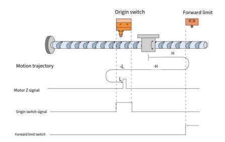
When HOME=OFF, POT=OFF, it starts to homing at high speed in the forward direction. After encountering the rising edge of POT, it automatically runs in the reverse direction at high speed. After encountering the rising edge of HOME, it runs in the reverse direction at low speed. After encountering the falling edge of
