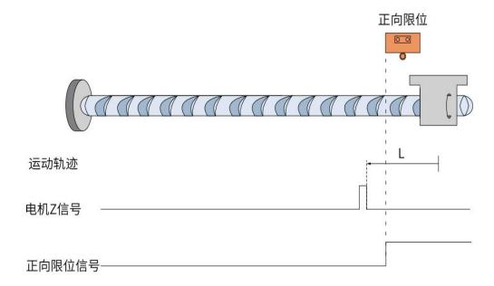
When POT=ON, it starts homing, directly reverse homing at low speed, and stops at the first Z signal after encountering the falling edge of POT.
