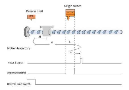
When HOME=OFF, NOT=OFF, it starts homing at high speed in the reverse direction. After encountering the rising edge of NOT, it immediately runs in the
