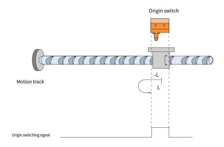
When HOME=ON, it starts homing at a low speed in the reverse direction. After encountering the falling edge of NOT, it decelerates and reverses, runs at a low speed in the forward direction, and stops after encountering the rising edge of HOME.
