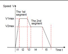
V1max, V2max: the first and second segment command speeds;
