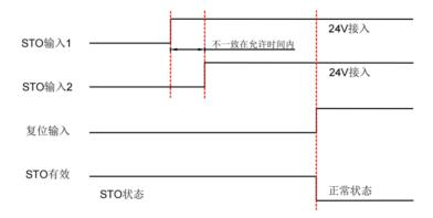
Note: The servo can be enabled or disabled only after the STO status exits normally.
