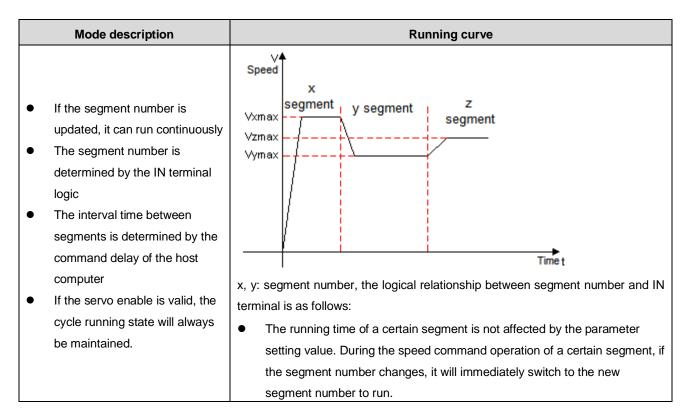
When the multi-segment position operation mode is set to IN switching operation, please configure the 4 IN terminals of the driver as functions 14~17 (FunIN.14~FunIN.17: multi-segment running command switching), and confirm the valid logic of IN terminal. At the same time, one IN terminal of the servo driver can be configured as function 19 (FunIN.19: speed command direction setting) to switch the speed command direction.
