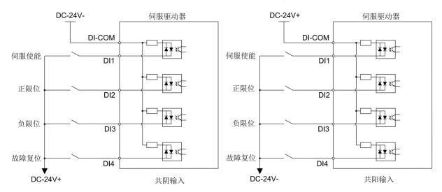
Take IN1 as an example, the wiring example is as follows:
