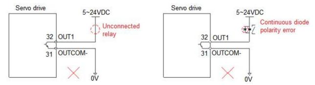
(2) When the upper device is optocoupler input
