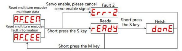
Note: When using this operation, please disable the servo enable signal, otherwise the fault information cannot be reset.
