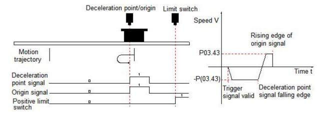
3) The origin switch (decelerate point) signal is invalid (0 - invalid, 1 - valid) before the motor returns to origin, and the positive limit switch is triggered during the process of returning to origin.
