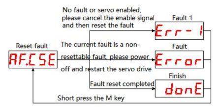
Note: When using this operation, please disable the servo enable signal, otherwise the fault information cannot be reset.
