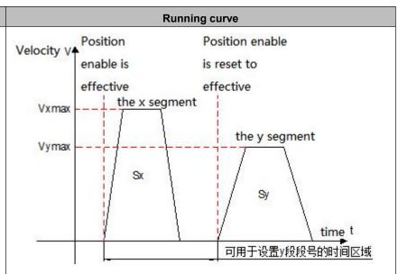
Vxmax. Vymax: Maximum operating speed of the x-th and y-th segment Sx. Sy: The x-th segment and the y-th segment displacement
