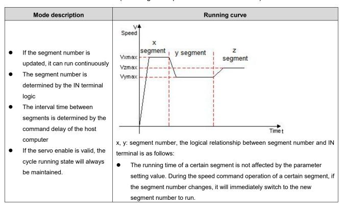
When the multi-segment position operation mode is set to IN switching operation, please configure the 4 IN terminals of the drive as functions  $14\sim17$  (FunIN.14 $\sim$ FunIN.17: multi-segment running command switching), and confirm the valid logic of IN terminal. At the same time, one IN terminal of the servo drive can be configured as function 19 (FunIN.19: speed command direction setting) to switch the speed command direction.
