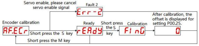
◆ Note: When using this operation, please disable the servo enable signal.
