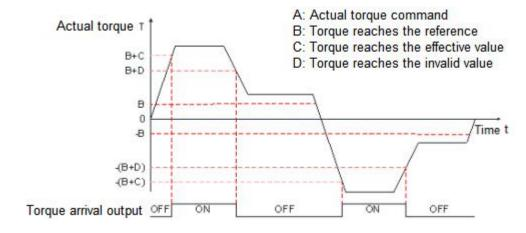
Actual torque command (The value of parameter P13.03 can be read by communication):
