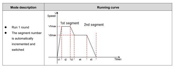
V1max、V2max: Command speed of the 1st and 2nd segment.
