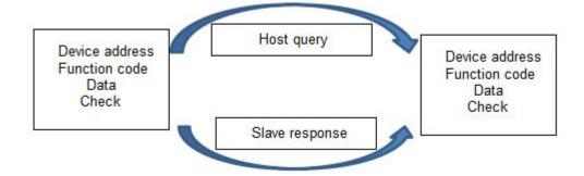
◆ Note: The communication data frame structure of this servo drive adopts RTU mode.
