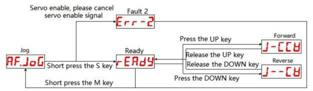
Note: When using this operation, please disable the servo enable signal.
