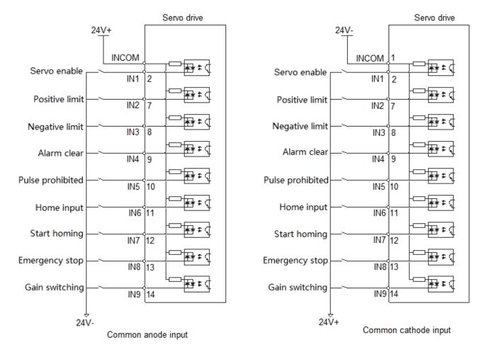
Take IN1 as an example, the wiring example is as follows:
