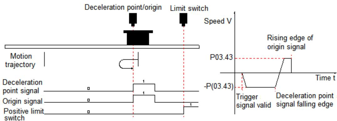
③ The origin switch (decelerate point) signal is invalid (0 - invalid, 1 - valid) before the motor returns to origin, and the positive limit switch is triggered during the process of returning to origin.
