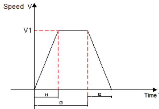
As shown in the figure above, the speed command of this segment is V1, and the actual acceleration time t1 is:
