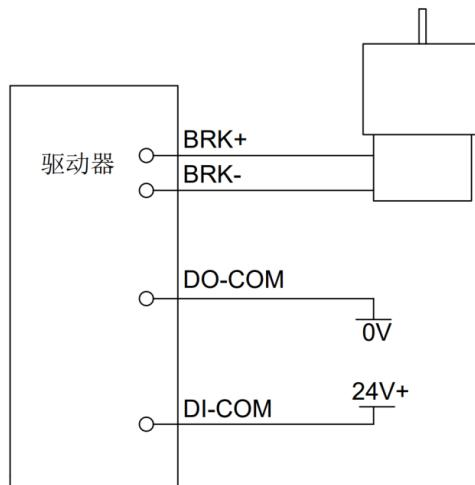
(2) For a common cathode DI input (where DI-COM is connected to 0V), the brake connection is as follows:
