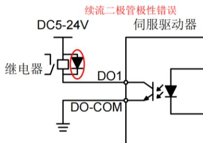
(2) When the upper device is optocoupler input
