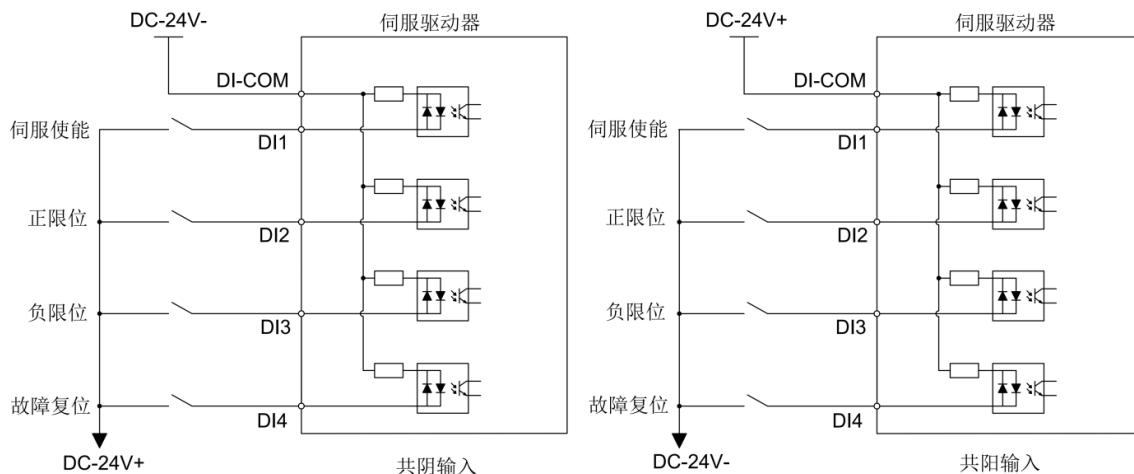
Take DI1 as an example, the wiring example is as follows:
