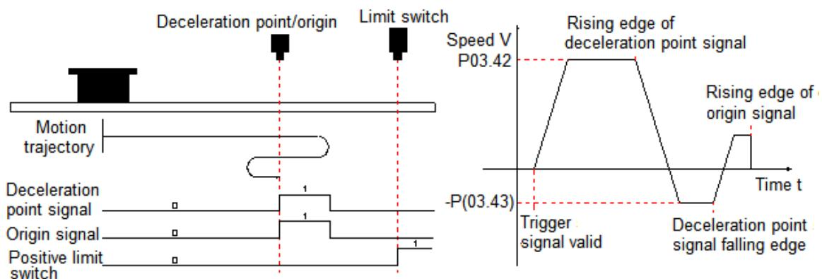
② The origin switch (decelerate point) signal is valid (0 - invalid, 1 - valid) before the motor returns to origin, and the positive limit switch is not triggered in the whole process.
