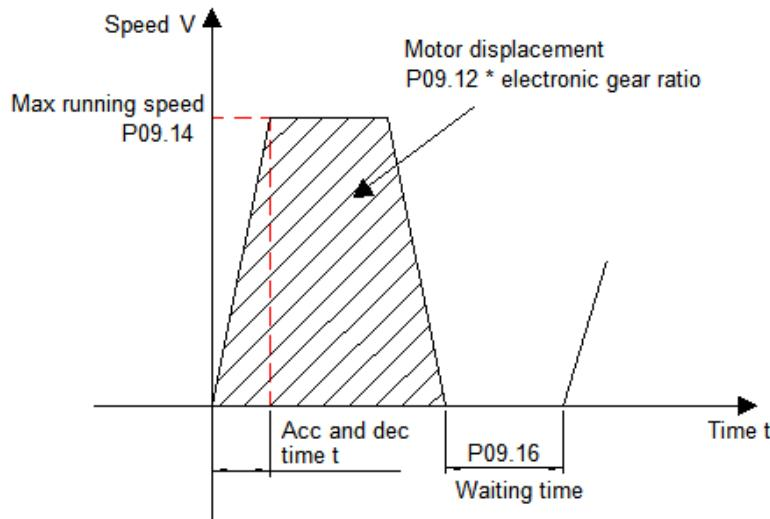
Therefore, the actual acceleration time  $t$  to P09.14 (Maximum running speed of segment 1 displacement):
