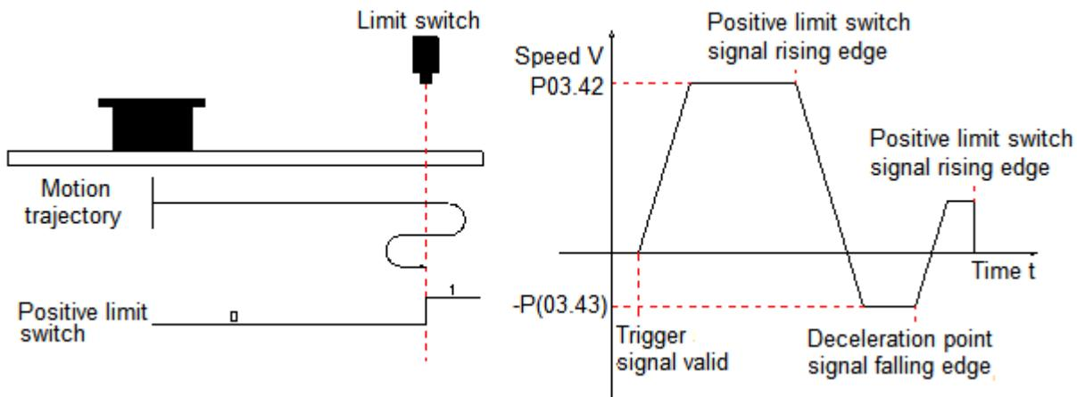
**② Positive limit switch (deceleration point) signal is valid (0 - invalid, 1 - valid) before the motor returns to origin.**
